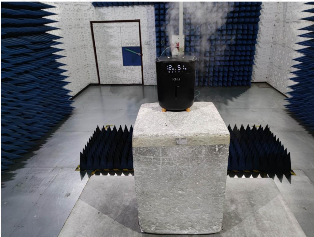
RADIATED EMISSION TEST SETUP ABOVE 1GHZ
