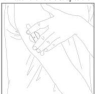
3. Attach the metal ring to the transmitter and peel off the double-sided adhesive release paper from the ring.
