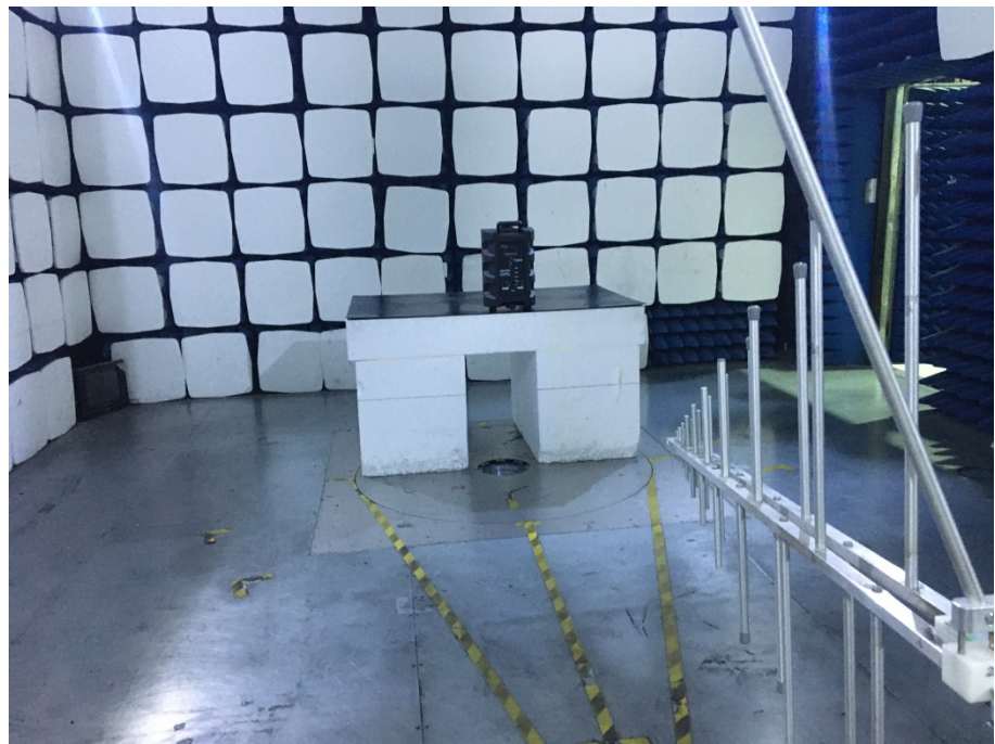
Radiation Emission Test Setup (30MHz to 1GHz)
