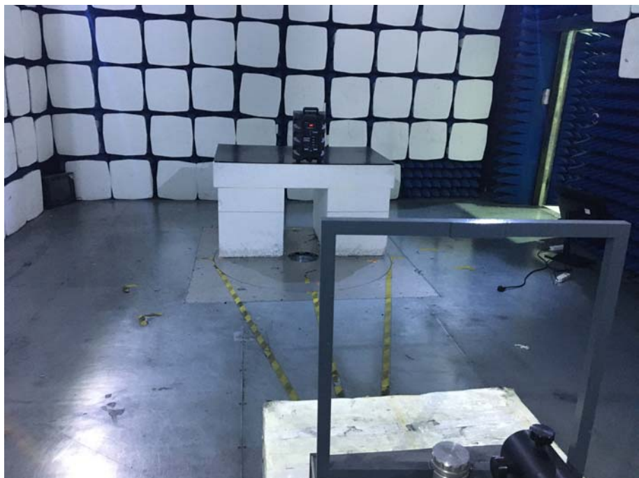
Radiation Emission Test Setup (Below 30MHz)
