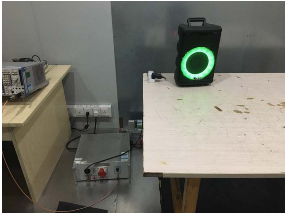
Conducted Emission Test Setup
