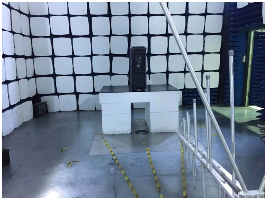
Radiation Emission Test Setup (30MHz to 1GHz)
