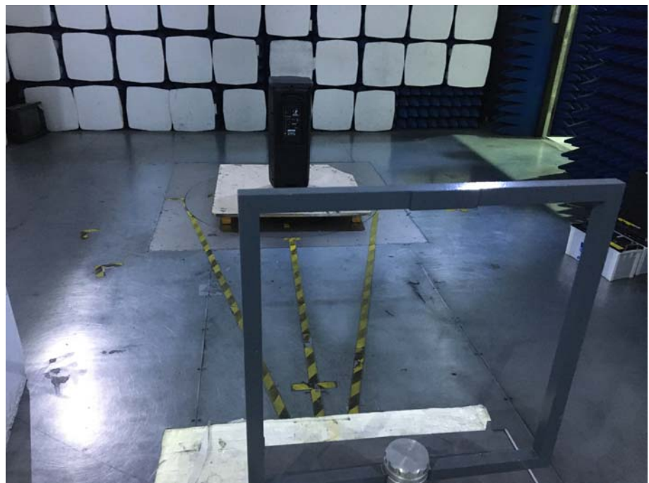
Radiation Emission Test Setup (Below 30MHz)
