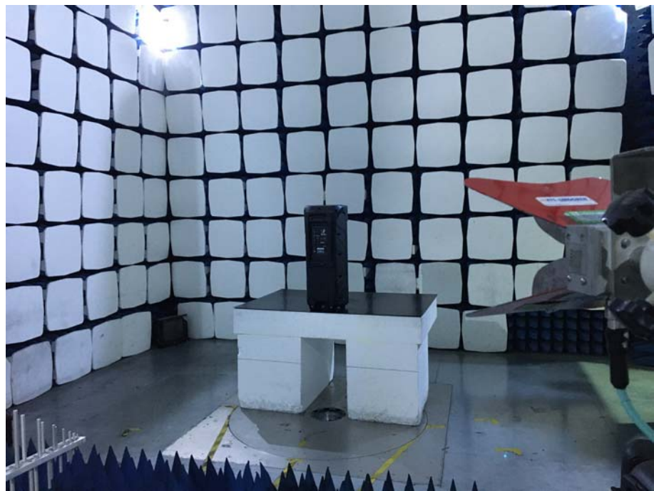
Radiation Emission Test Setup (1GHz to 18GHz)
