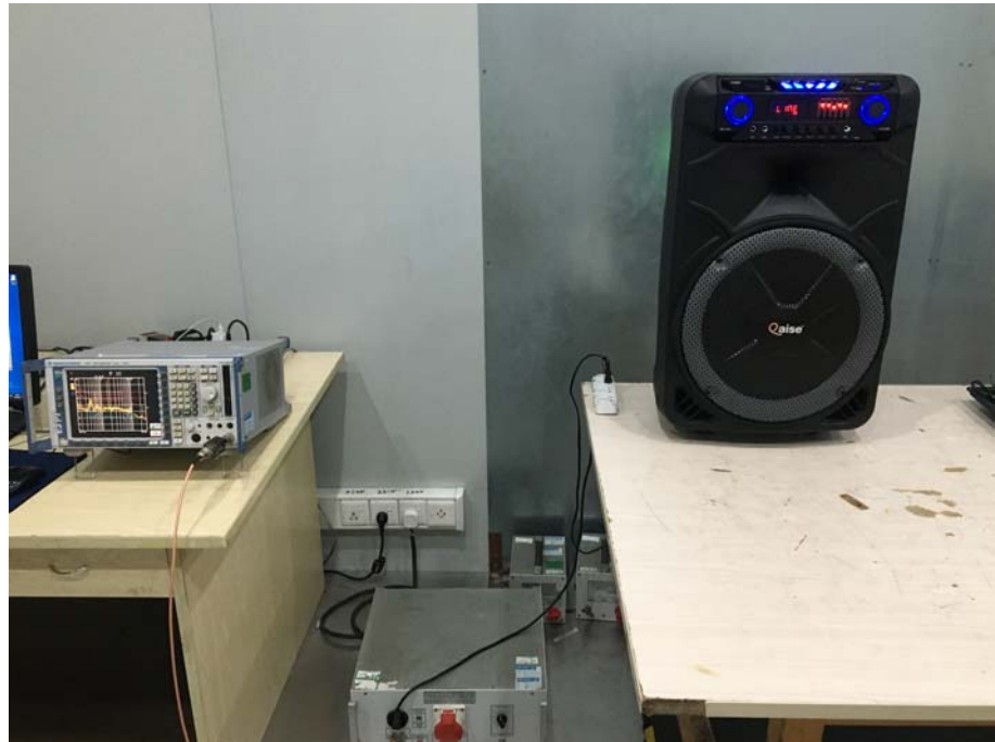
Conducted Emission Test Setup
