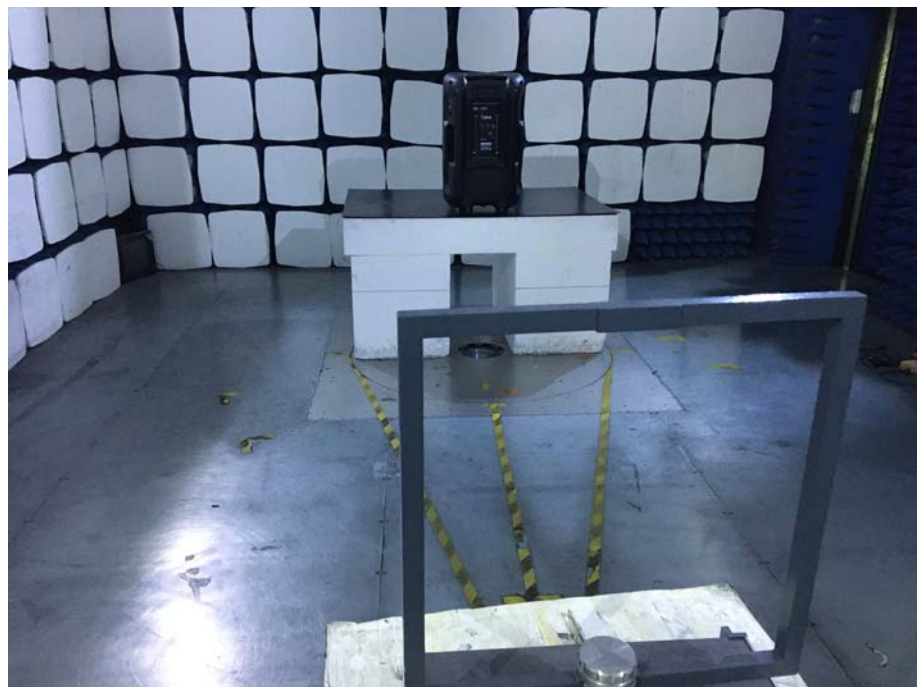
Radiation Emission Test Setup (Below 30MHz)
