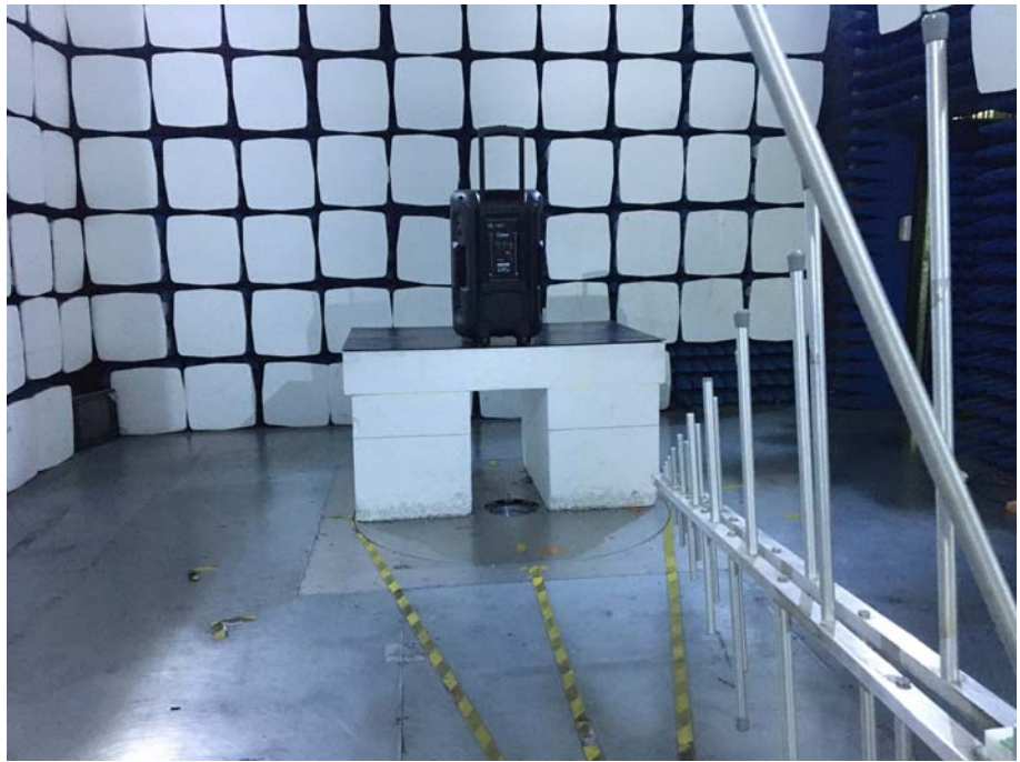
Radiation Emission Test Setup (30MHz to 1GHz)
