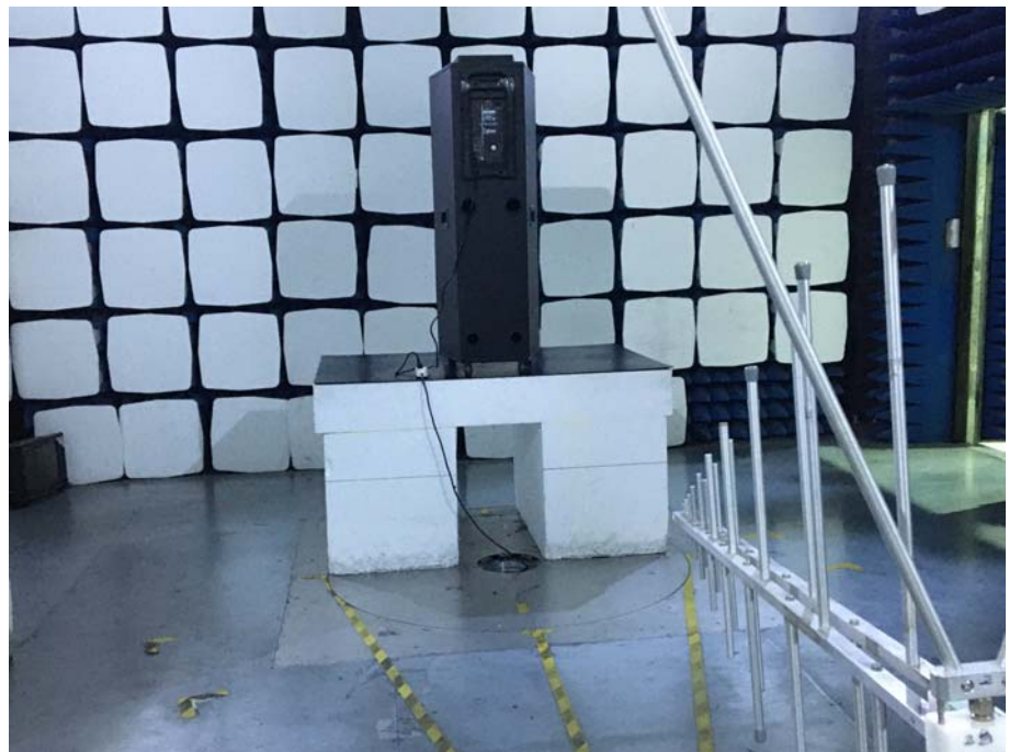
Radiation Emission Test Setup (30MHz to 1GHz)
