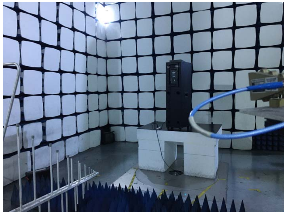
Radiation Emission Test Setup (Above 18GHz)
