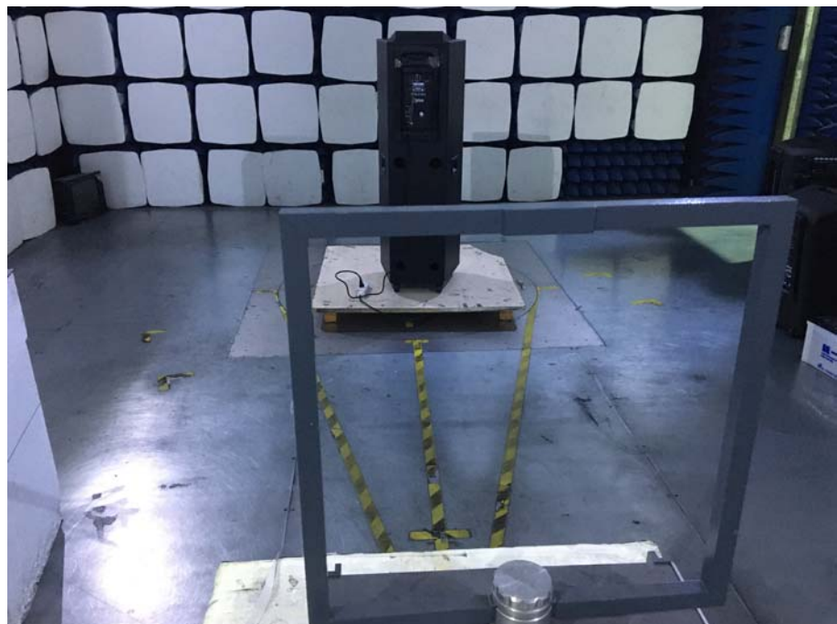
Radiation Emission Test Setup (Below 30MHz)
