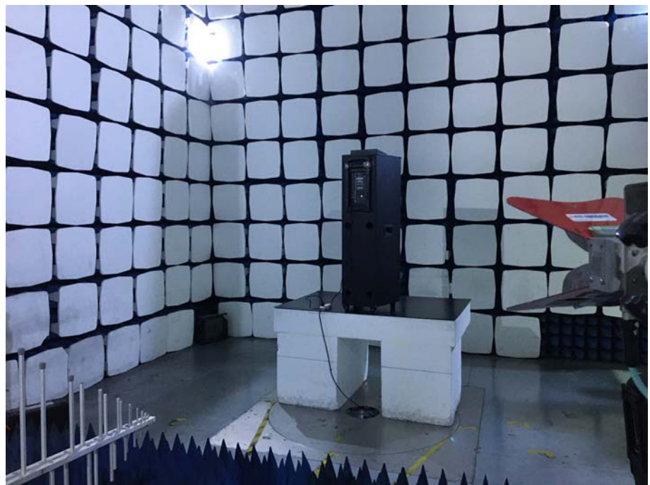
Radiation Emission Test Setup (1GHz to 18GHz)
