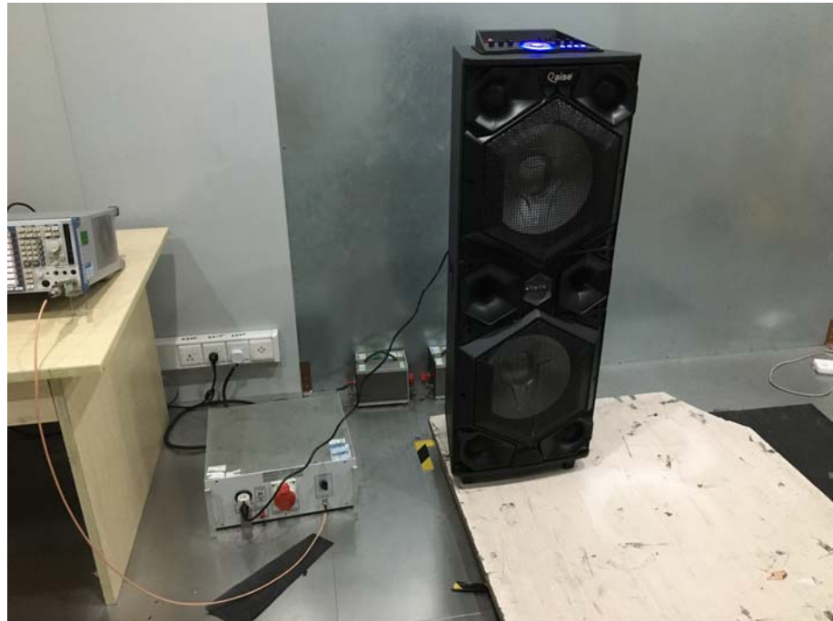
Conducted Emission Test Setup
