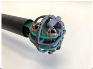
Test probe, without the casing
