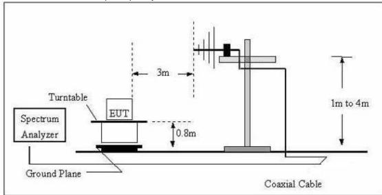
(C) Radiated Emission Test-Up Frequency Above 1GHz
