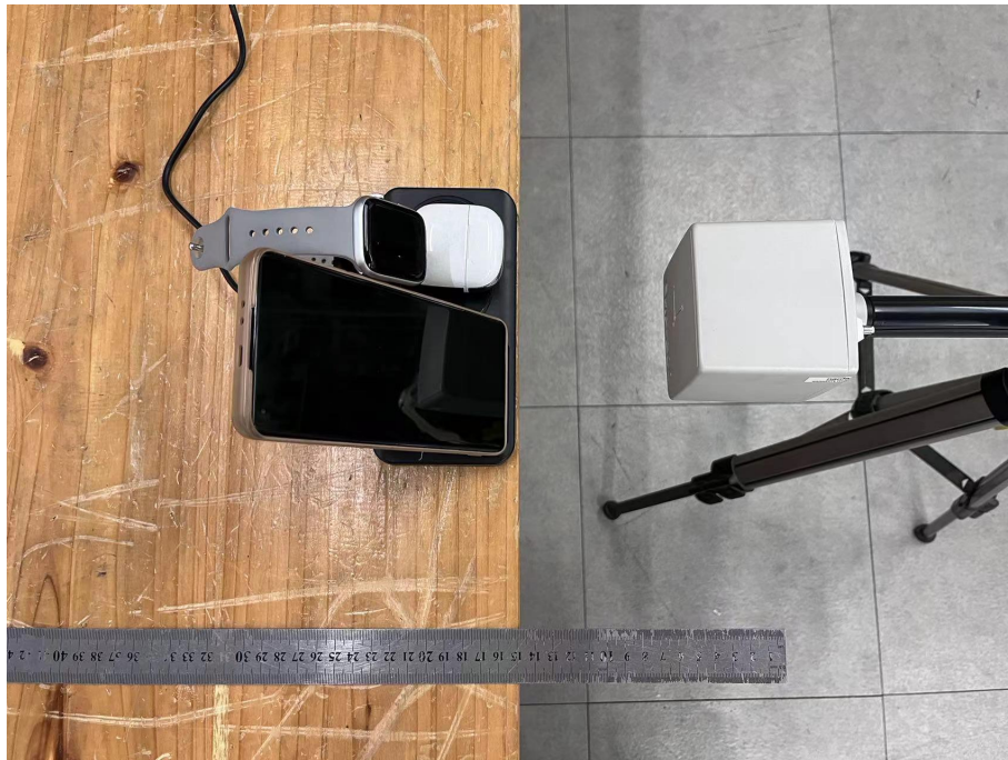
Test Position A-15cm from the edge of EUT to the geometric center of the probe
