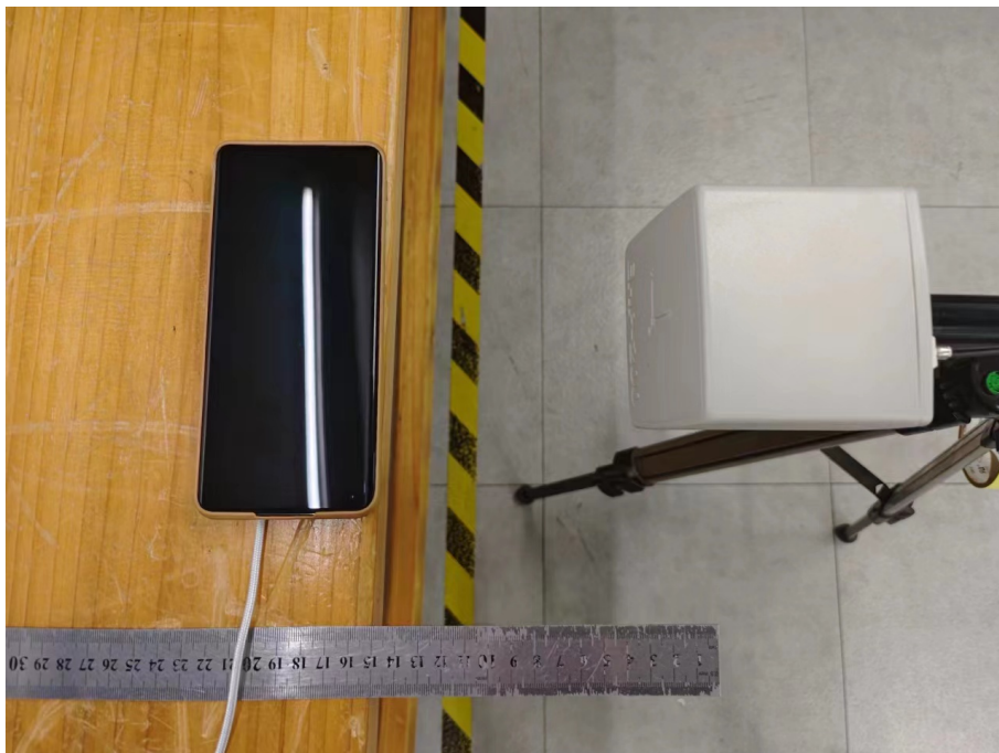
Test Position D-15cm from the edge of EUT to the geometric center of the probe
