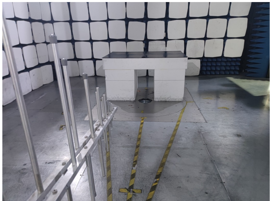
Radiation Emission Test Setup (30MHz to 1GHz)
