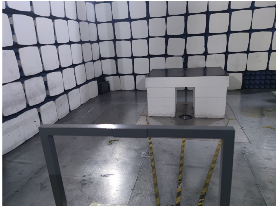
Radiation Emission Test Setup (Below 30MHz)
