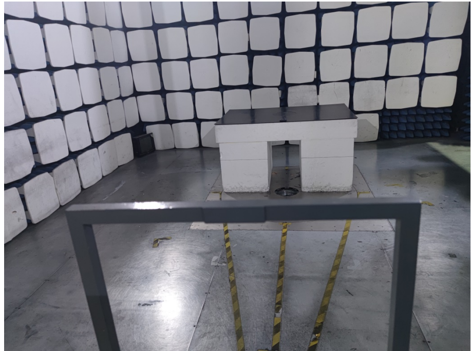
Radiation Emission Test Setup (Below 30MHz)
