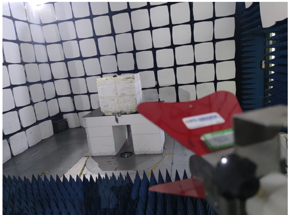
Radiation Emission Test Setup (1GHz to 18GHz)
