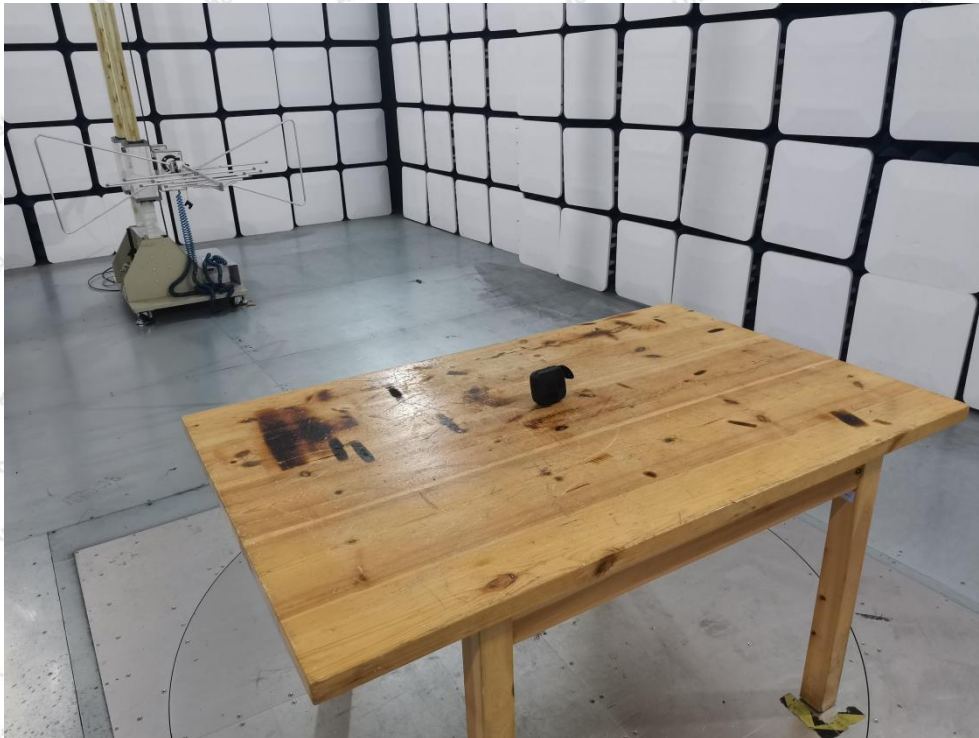
Photo of Radiation Emission Test
