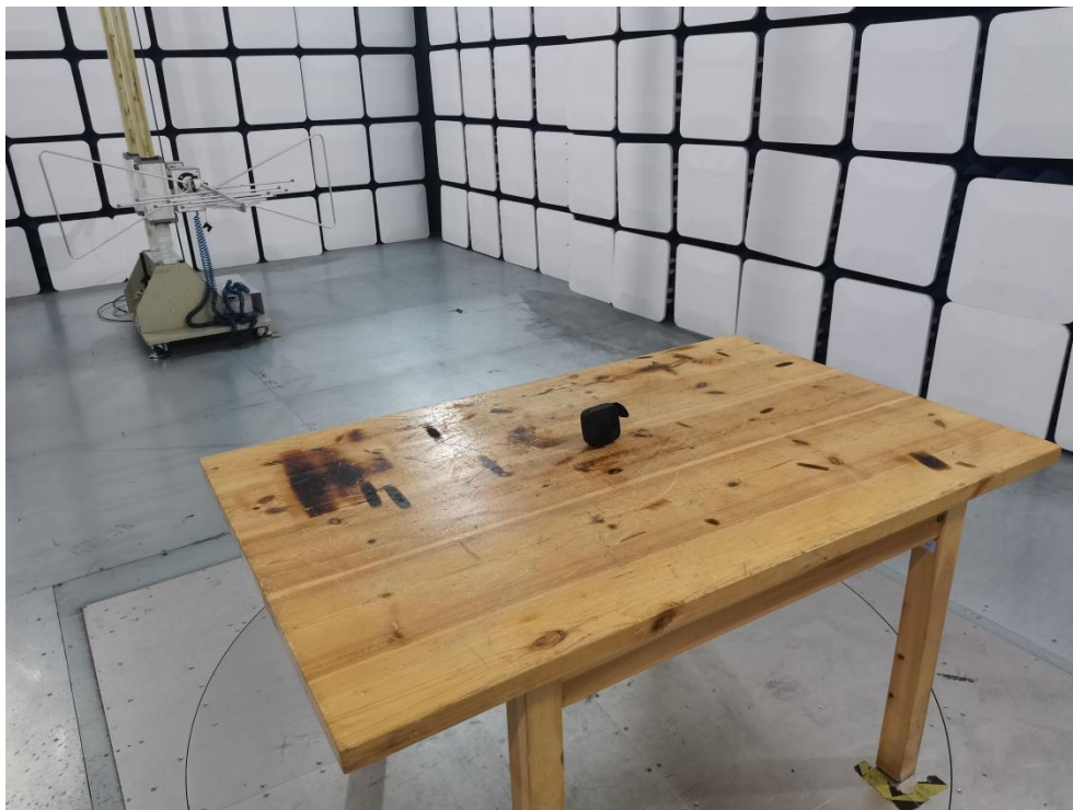
Photo of Radiation Emission Test
