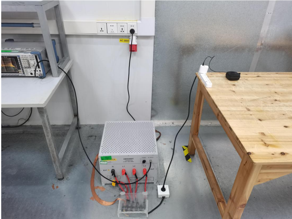
Photo of Conducted Emission Measurement
