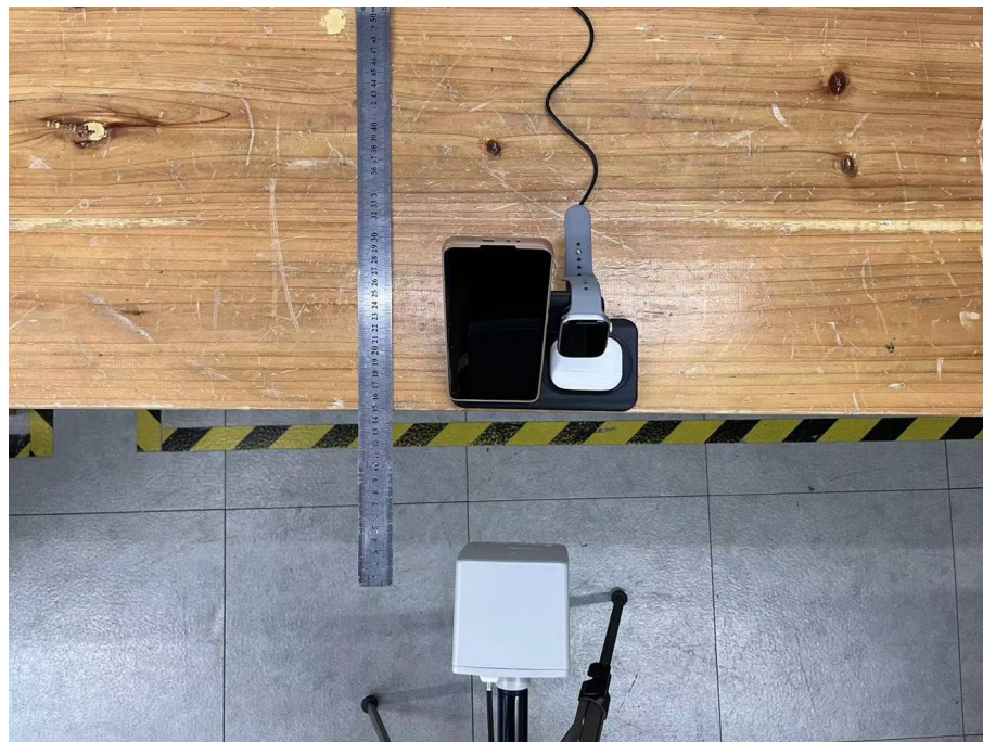
Test Position B-15cm from the edge of EUT to the geometric center of the probe
