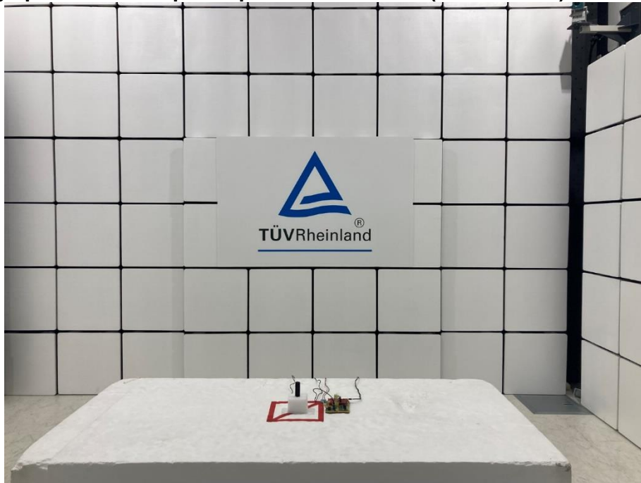
Photograph 2: Test Setup for Spurious Emissions (Front View 2)
