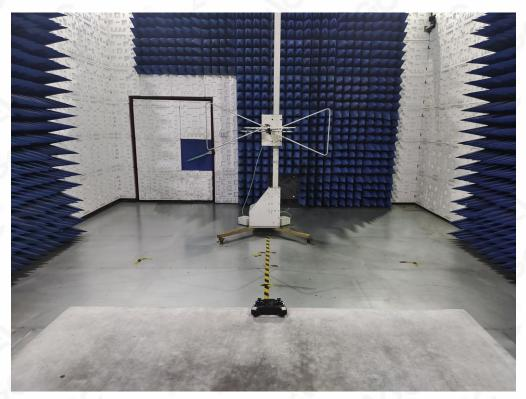
RADIATED EMISSION TEST SETUP ABOVE 1GHz
