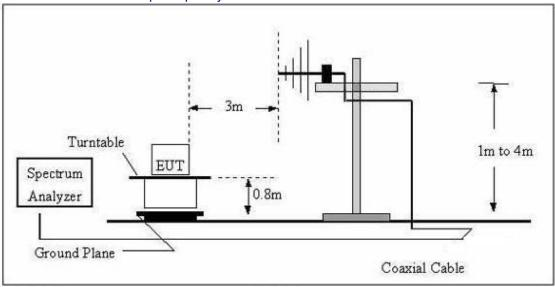
(C) Radiated Emission Test-Up Frequency Above 1GHz
