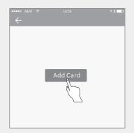
There are three options for you. Select "permanent", "timed" or "recycling" as needed. Enter the name of the RFID card, and click "OK". Then, when the RFID card is close to the card sensing area of the lock for 2-3 seconds, the RFID card can be added successfully.
