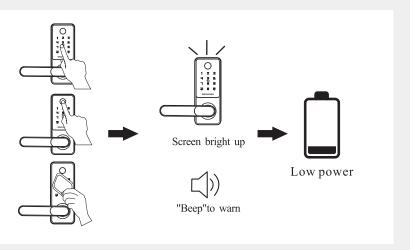
When the smart lock is open, the screen will brighten up and "beep" to warn that the battery is low power.
