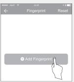
There are three options for you. Select "permanent", "timed" or "recycling" as needed. Enter the name of the Fingerprint, and click "OK". Then click "Start" and you will be required to place and remove your finger from the sensor 4 times.
