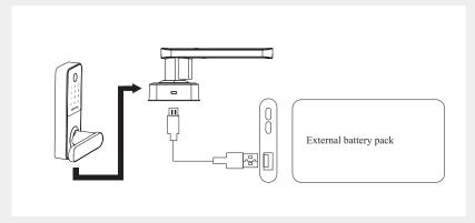
If the lock is low power and unable to operate, there is a micro USB power socket at the bottom of lock for power supply.
