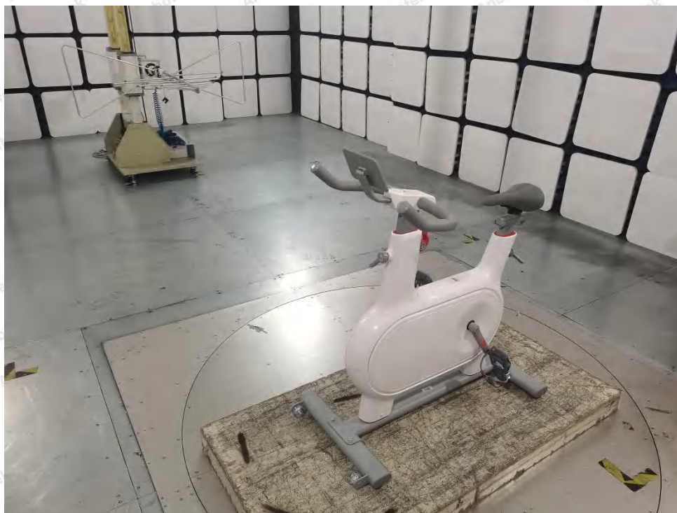
Photo of Radiation Emission Test
