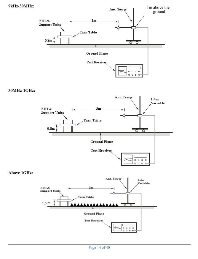
The radiated emissions were performed in the 3 meters distance, using the setup accordance with the ANSI C63.10-2013. The specification used was the FCC 15.205, 15.209, and FCC 15.231 limits.
