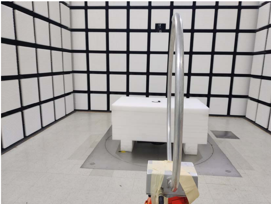
9kHz~30MHz_Radiated Emission View Perpendicular
