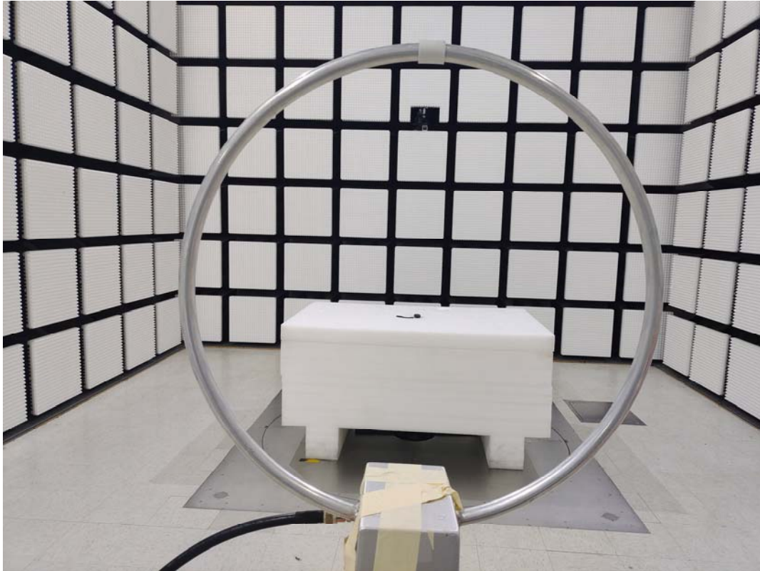
9kHz~30MHz_Radiated Emission View Perpendicular
