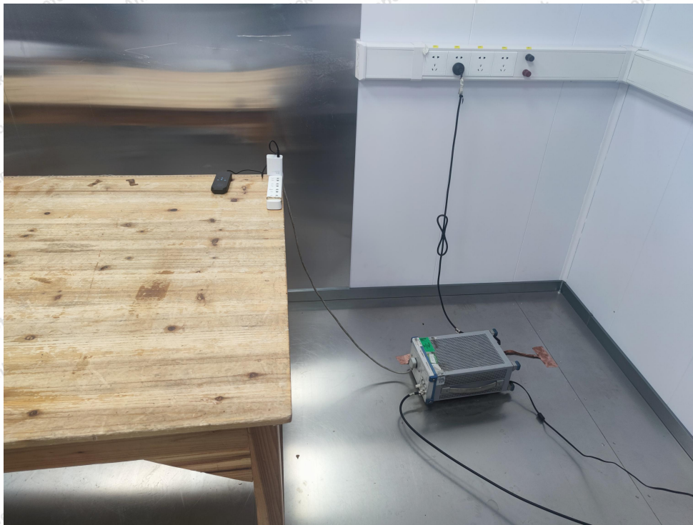
Photo of Conducted Emission Measurement
