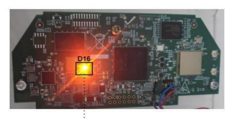
When board is powered ON D16 LED (in top of mesh card)will glow
