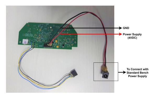
The Mesh card needs to be powered with the 4V supply from a **Standard bench power supply** using the cable assembly with DC Jack which should be connected to the IO Connector J5 on the board as shown in the above image.
