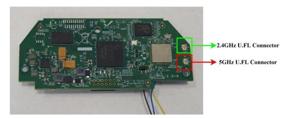
The 11n Mesh card supports WiFi 2.4GHz and 5GHz Radios. The dual band patch antenna is used and needs to be connected with the on-board U.FL connectors highlighted in the above image.
