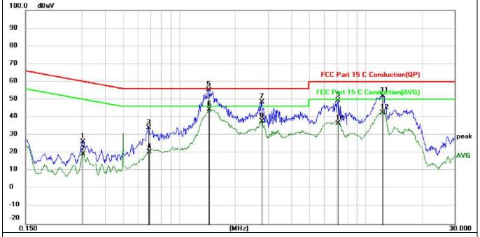
Remark: Factor = LISN factor + Cable Loss + Pulse limiter factor.
