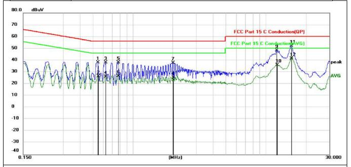
Remark: Factor = LISN factor + Cable Loss + Pulse limiter factor.
