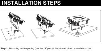
Step 1: According to the spacing (see the "A" part of the picture) of two screw bits on the LED Light bracket, drill two mounting holes.
