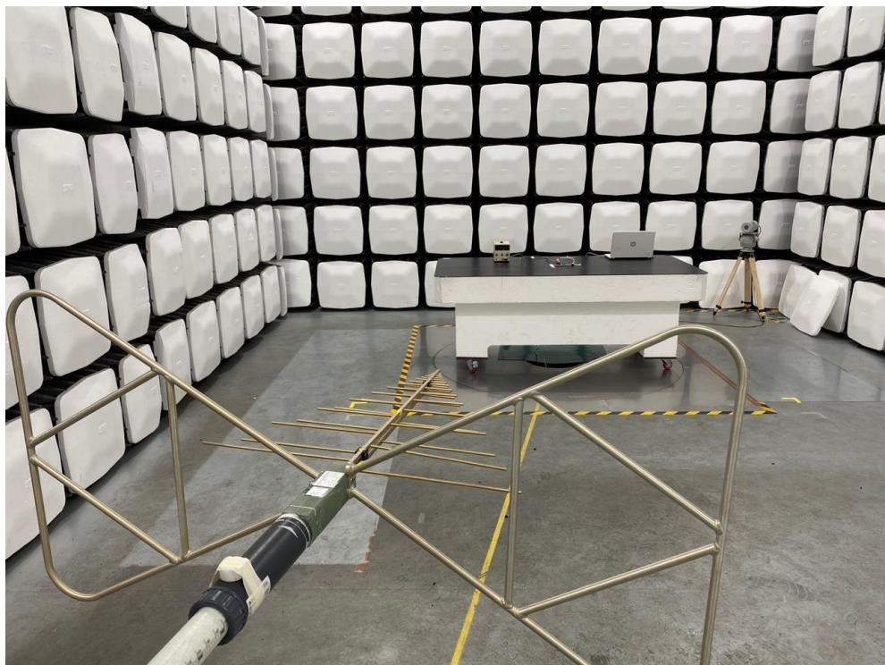
**- Radiated Emission Test (Above 1 GHz)**
