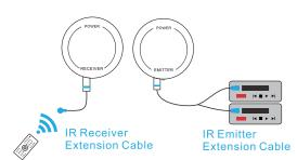
**Step One:** If you want to extend the reach or hide the IR receiver, connect the IR Receiver Extension Cable to the device.
