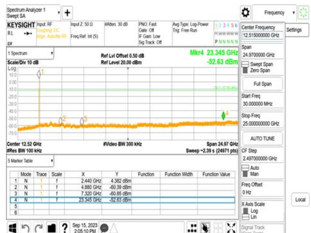
Spurious Emission_BLE 1M_MidCH19-2440MHz
