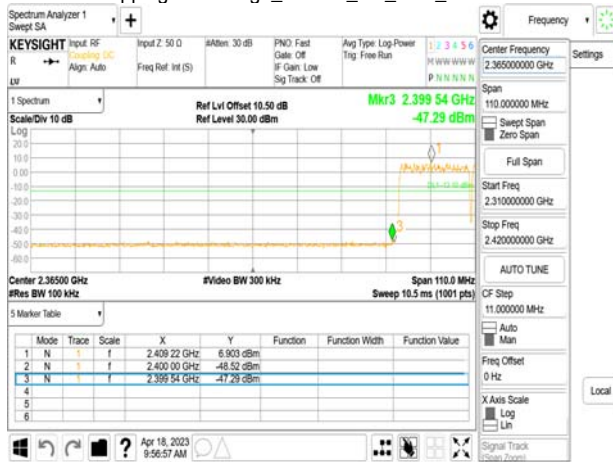
Hopping Band Edge_8DPSK_3M_DH5_2480MHz
