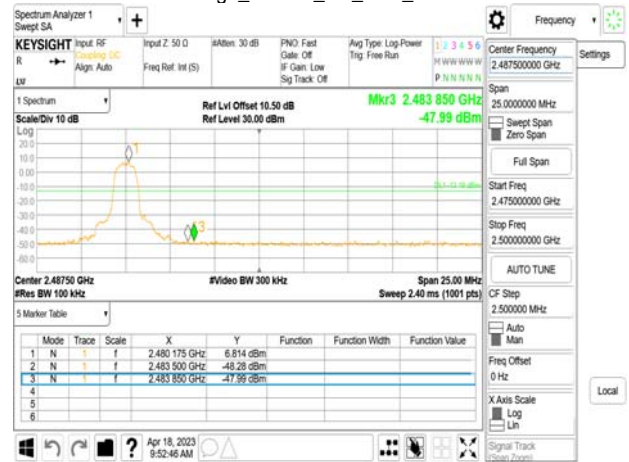
Hopping Band Edge_GFSK_1M_DH5_2402MHz
