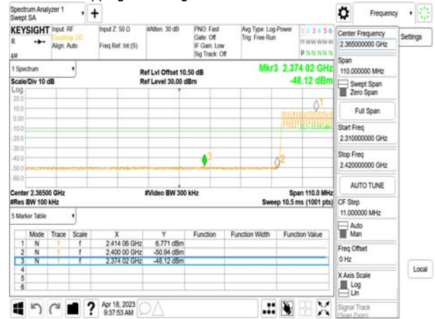
Hopping Band Edge_GFSK_1M_DH5_2480MHz
