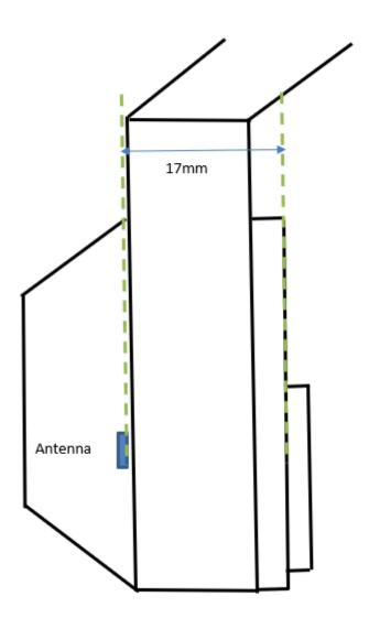
Min. distance from antenna to human body measured: 17mm
