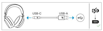
1. Make sure that the charging socket if free from moisture and contamination. Connect the USB-C connector of the charging cable to the USB socket of the headphones.
