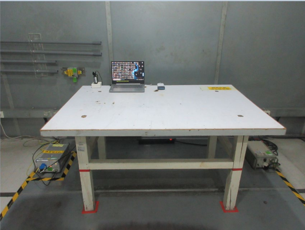
AC Power Line Conducted Emissions Test Photos
