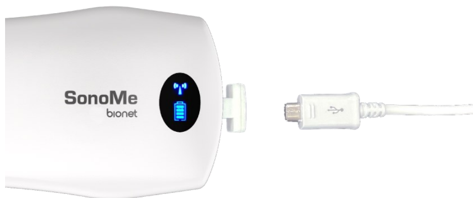
[Figure 4-1] Probe Charging via USB Cable
