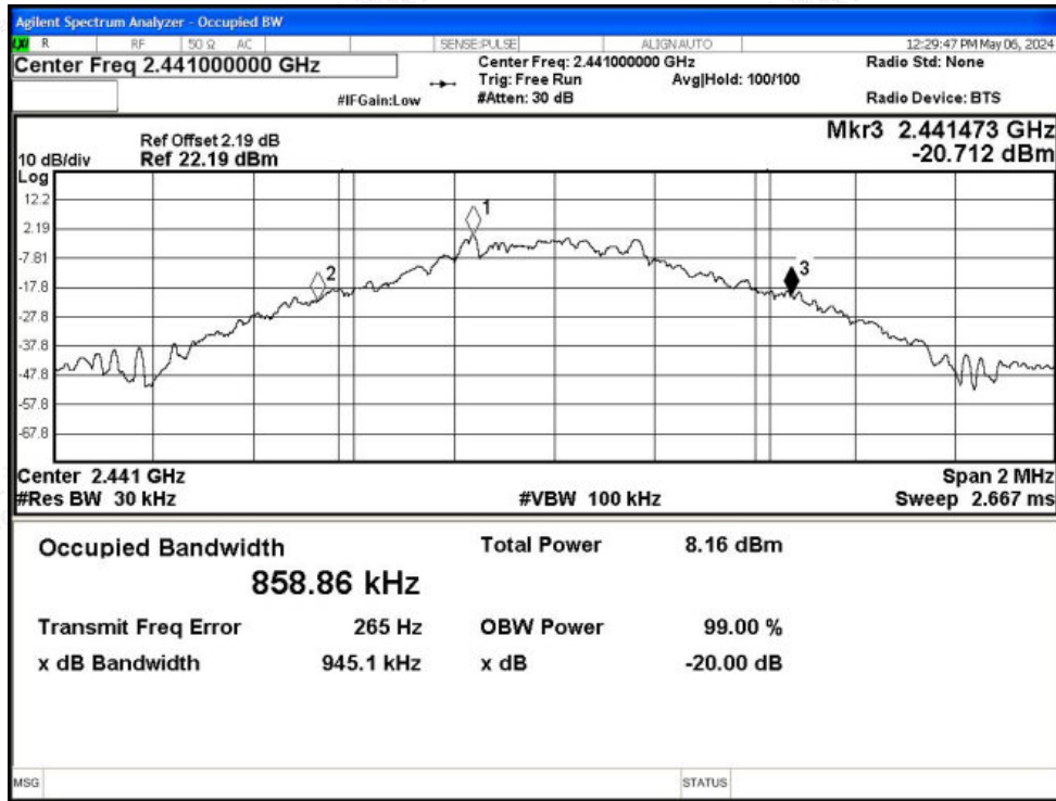
-20dB Bandwidth NVNT 1-DH5 2441MHz Ant1
