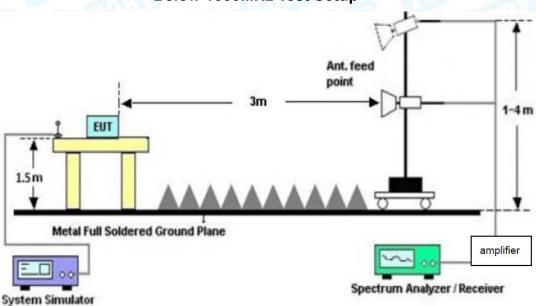
**Above 1GHz Test Setup**
