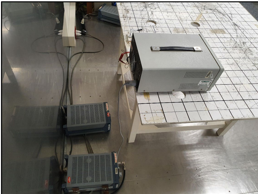
Photo 20 AC Conducted Test Setup- EUT+ Internal Antenna
