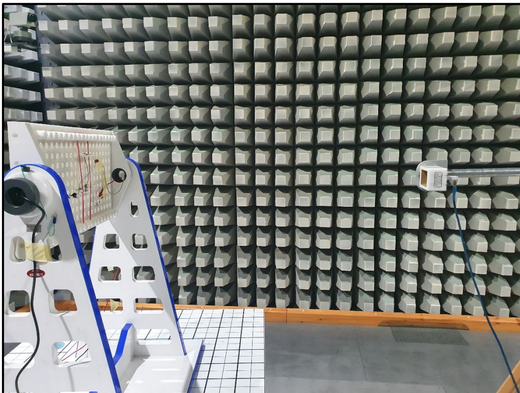
Photo 16: Radiated Test Setup - 18 GHz – 26.5 GHz - EUT+ External Antenna
