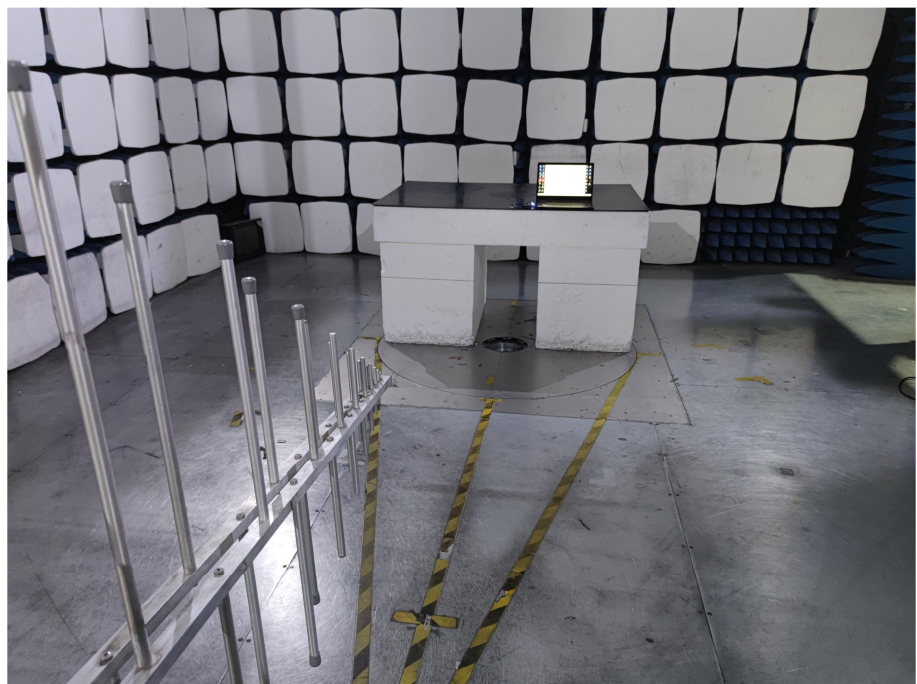
Radiation Emission Test Setup (30MHz to 1GHz)
