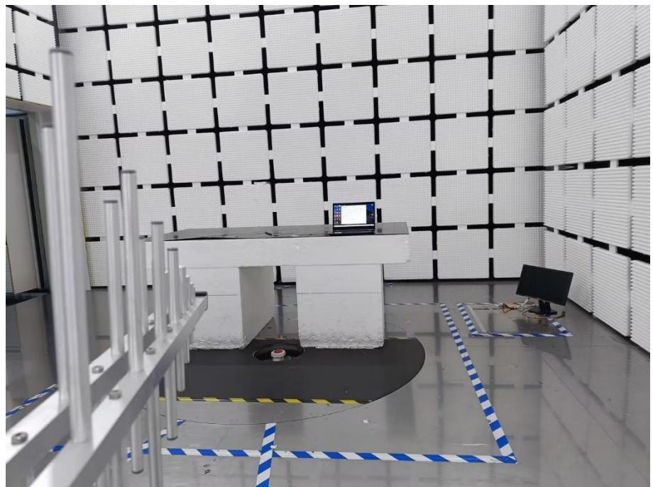
Radiation Emission Test Setup (30MHz to 1GHz)
