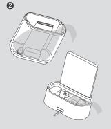
Drain any remaining water from the tank and the base.
