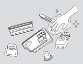
Clean all parts with a soft cloth, you may use the included cleaning brush to remove excess of mineral deposit. Make sure all parts are dry before reassembling your humidifier.
