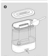
Fill the tank with a solution of citric acid and water (one teaspoon of citric acid for each gallon of water). Replace the tank cover and shake around the tank.
