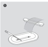
Detach the water tank from the base. Take out the water tank cover and rinse it with warm water.
