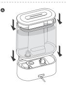
Put the water tank back in place and close the top cover.
