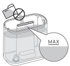
Fill the tank with water, making sure the water doesn't pass the MAX line.
