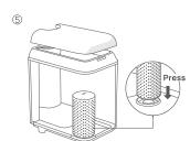
Attach the demineralization cartridge to the tank. If your humidifier doesn't include it, replace back the original filter.
