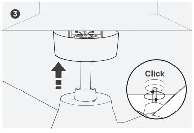
Rotate the canopy clockwise to securely fasten it to the ceiling bracket (You will hear a "click").
