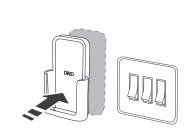
Peel off the 3M glue on the back of the holder to adhere it to the desired location.
