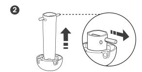
Lift the downrod upwards, then remove the horizontal bar, and detach the downrod ball from the 6-inch downrod.
