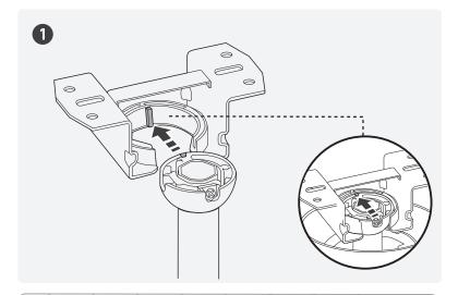
Place the downrod ball into the ceiling bracket.
