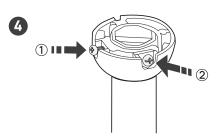
Insert the first perforated screw tightly, and then insert the second screw tightly.
