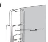
Align the two holes on the holder with the two holes on the wall.
