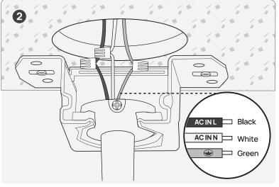
Connect the wires with matching colors from the ceiling fan body to the ceiling.
