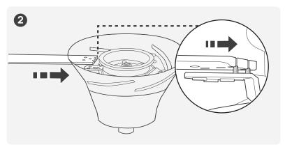
Make sure that the two blade slots align with the vertical tabs of the ceiling fan body.
