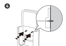
Insert the two screws into the holes and tighten them using a screwdriver.
