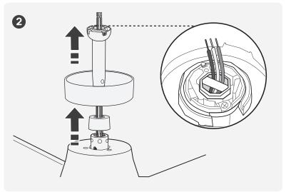
Pass all the wires to one side of the horizontal bar in the downrod to prevent excessive wire tangling.
