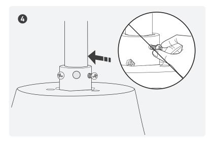
Tighten the setscrew with a screwdriver.
