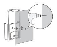
Use the two holes on the holder as a guide to drill two corresponding holes in the flat wall.
