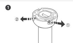
Loosen and remove the two screws on the downrod ball from the 6-inch downrod.
