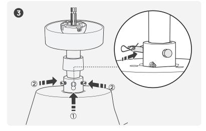
Slide the downrod into the yoke of the motor assembly,
