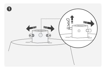
Remove the pre-installed setscrews and downrod pin from the downrod.
