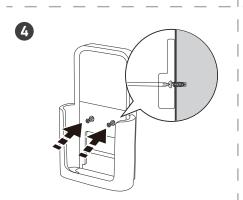
Insert the two screws into the holes and tighten them using a screwdriver.
