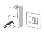
Peel off the 3M glue on the back of the holder to adhere it to the desired location.
