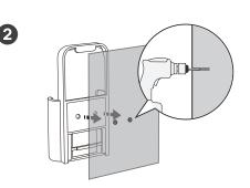
Use the two holes on the holder as a guide to drill two corresponding holes in the flat wall.
