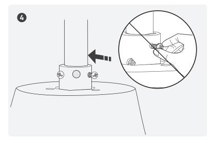
Tighten the setscrew with a screwdriver.
