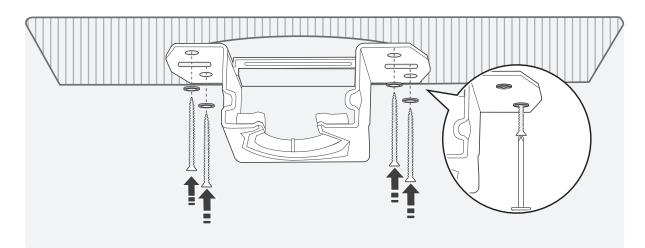
Option 1: Use wood screws when: Securing an approved electrical outlet box. Drill 9/64" pilot holes in support structure to aid in securing ceiling bracket.
