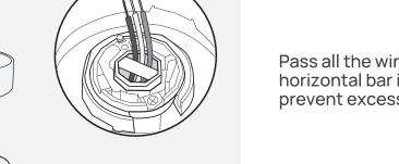
Pass all the wires to one side of the horizontal bar in the downrod to prevent excessive wire tangling.
