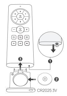
1. Unscrew the locking button with a Phillips screwdriver to remove the battery holder.
