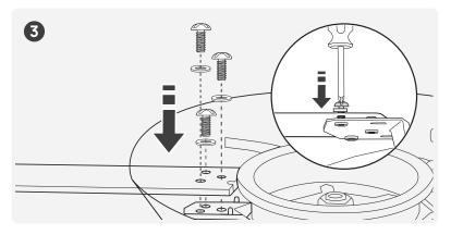
Partially insert the screws into the blade's holes, and then use a screwdriver to securely tighten them.
