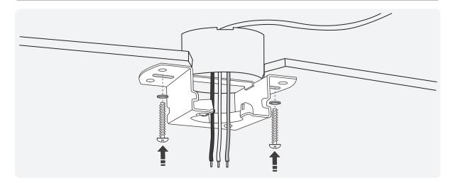
Option 2: Use machine screws (provided with outlet box) when: Securing to existing ceiling fan-rated outlet box. Make sure it is securely installed and is acceptable for fan support of 15.8kg (35 lbs) or less.
