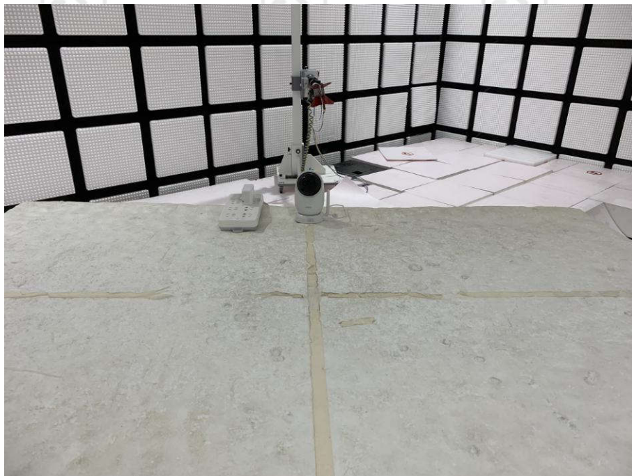
Radiated spurious emission Test Setup-2(1-18 GHz)
