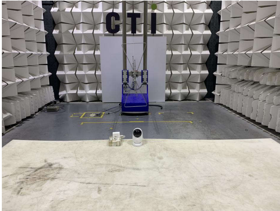
Radiated spurious emission Test Setup-1(Below 1GHz)
