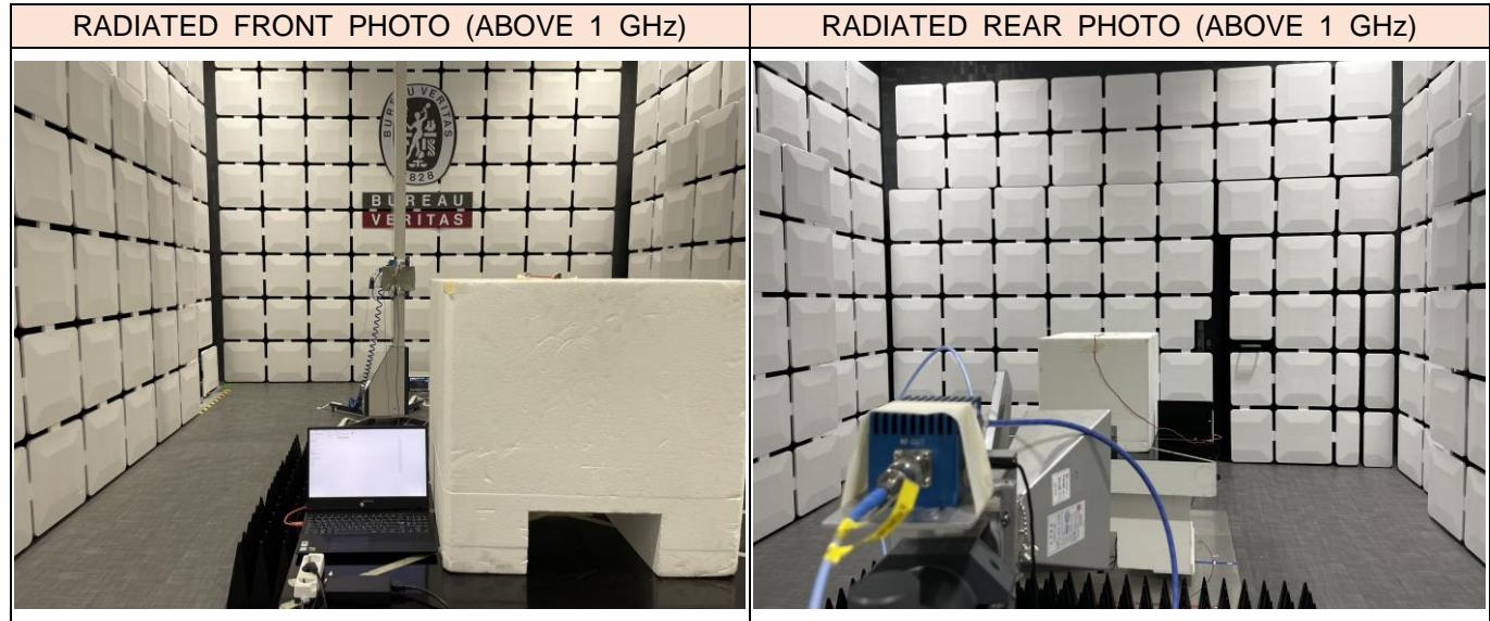
**RADIATED RF MEASUREMENT SETUP (18 - 26.5 GHz) Z axis**
