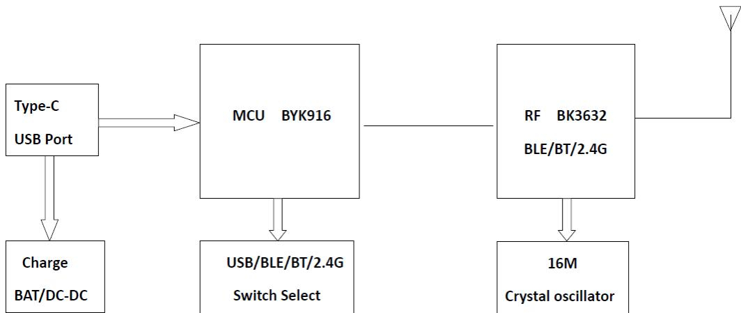
1. Cable mode 1-1, the wire mode USB-Type-C data cable from the host, the keyboard connected to a keyboard MCU BYK916 is to be sent when the USB-C data cable from the host command to send . 1-2, USB connection— Type-C data can also be charged to the battery .
