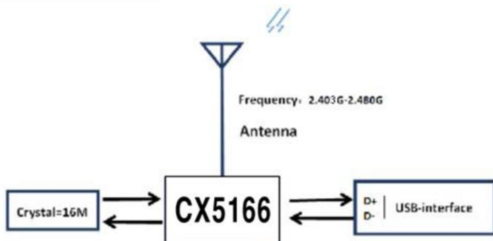
The receiver receives signals from the keyboard through the antenna, processes them by the MCU(CX5166), and transmits them to the computer via D+ and D- USB.
