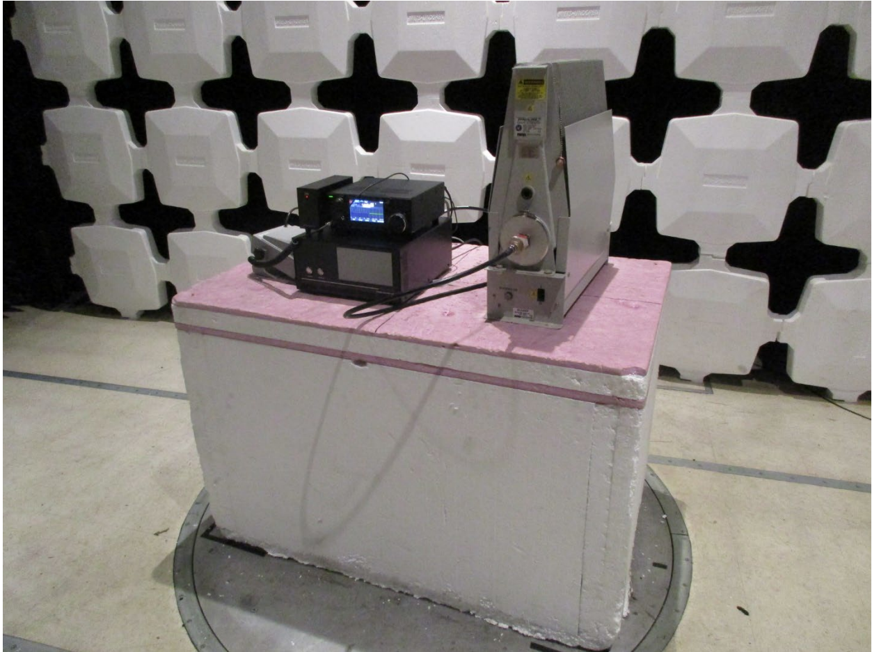
Radiated Testing, Table Setup
