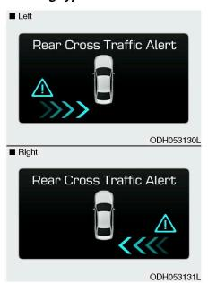
If the vehicle detected by the sensors approaches your vehicle, the warning chime will sound, the warning light on the outside rearview mirror will blink and a message will appear on the LCD display.
