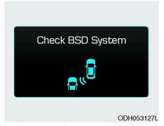
If the system does not work properly, a warning message will appear and the light on the switch will turn off. The system will turn off automatically. Have your vehicle checked by an authorized HYUNDAI dealer.
