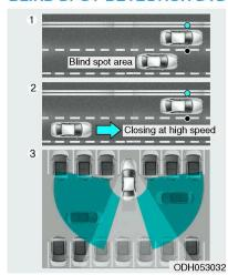
The Blind Spot Detection System (BSD) uses a radar sensor to alert the driver.
