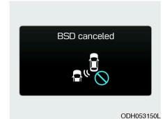
The message will appear to notify the driver if there are foreign substances on the rear bumper. The light on the switch and the system will turn off automatically.
