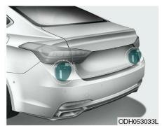
The sensors are located inside of the rear bumper.
