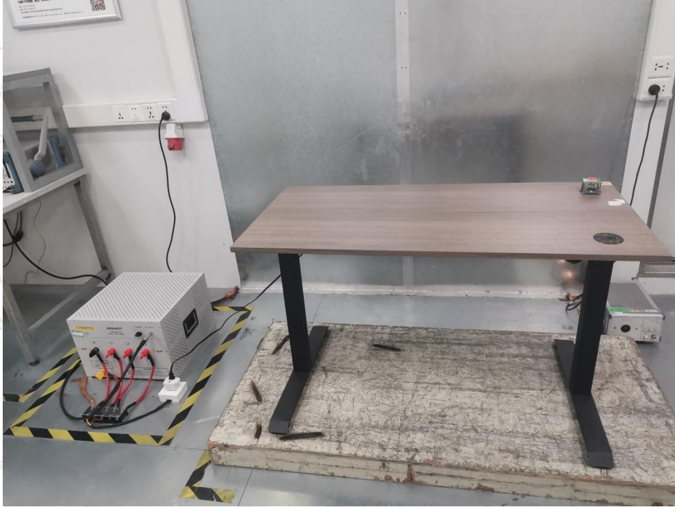
Photo of Conducted Emission Measurement
