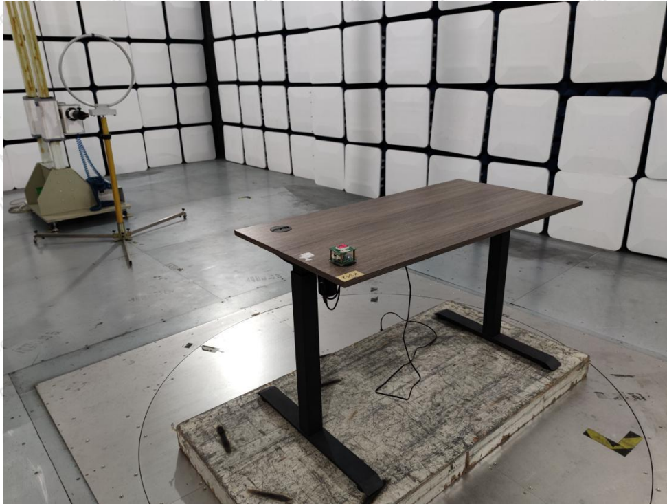
Photo of Radiation Emission Test
